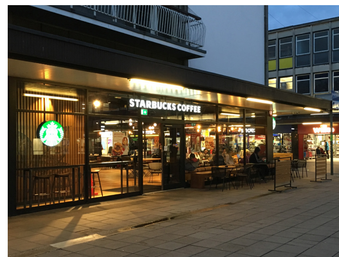
Example of successful shopfront with floor to ceiling glazing allowing long views into the shop unit, rationalised banner signage proportionate to the architectural and canopy scale and use of warm materials and lighting.
