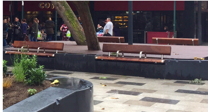
Feature elements in defined spaces should be designed to retain a degree of consistency with the standard palette. Above, a timber and granite plinth with integrated timber and stainless steel benches, matching the standard benches in finish and colour (Littlewood Square) or timber planters with integrated seating.
